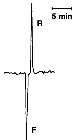
Figure 6 Separation of chiral components by HPLC with optical activity detection. Component F = fructose, component R = raffinose. Taken with permission from ref. 28.
